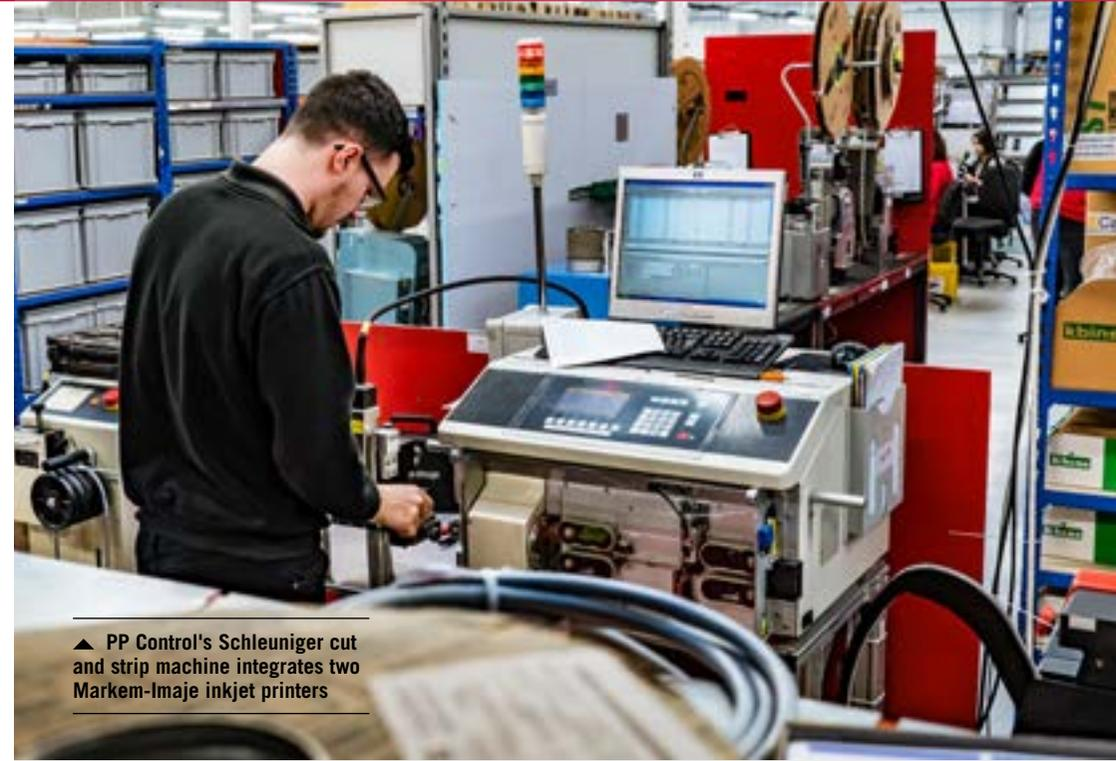
▲ PP Control's Schleuniger cut and strip machine integrates two Markem-Imaje inkjet printers
