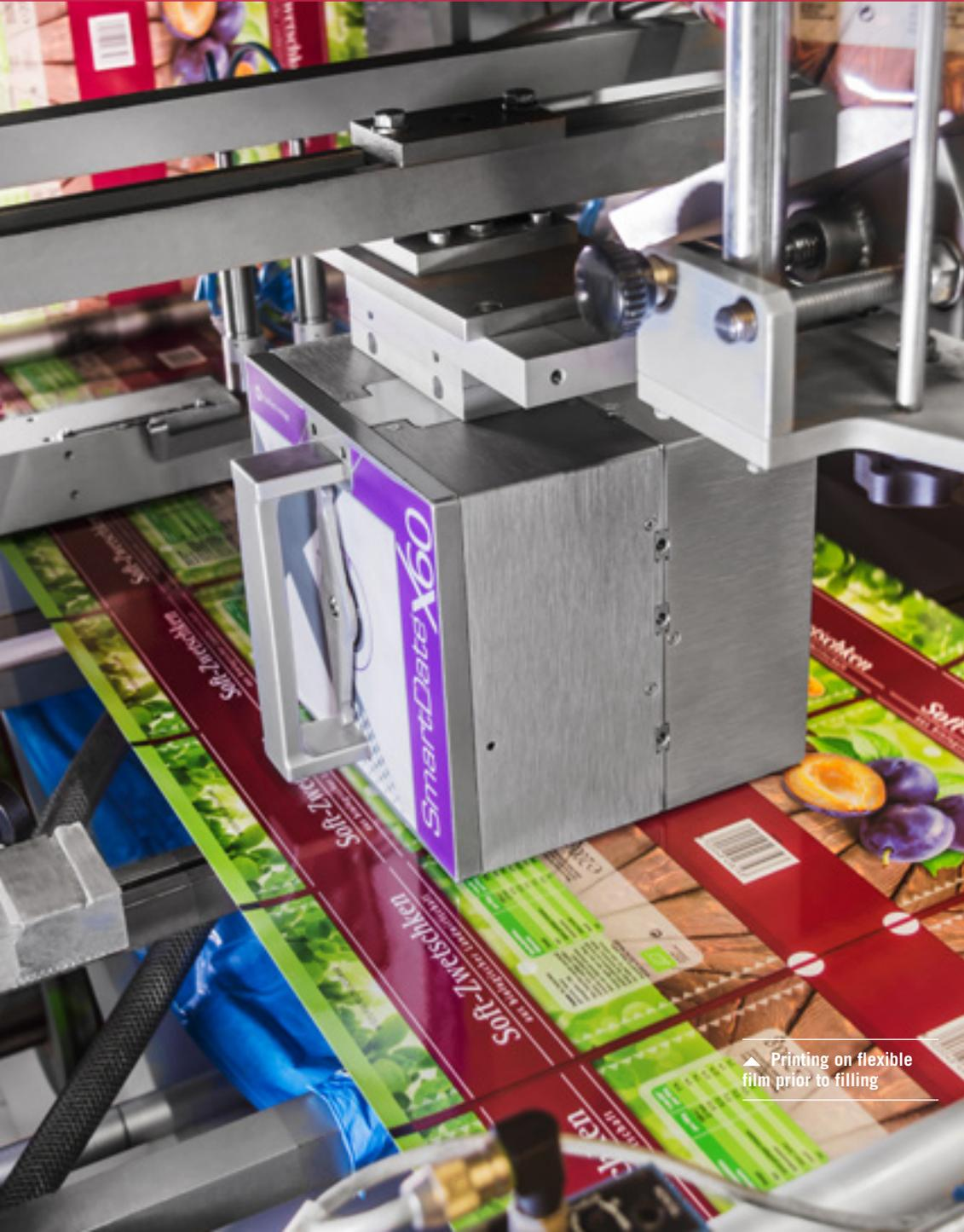
▲ Printing on flexible film prior to filling
